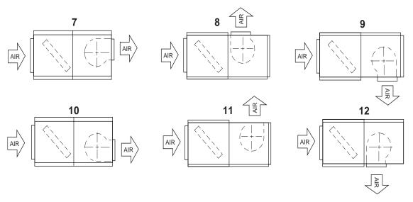
FIGURE 7 - HORIZONTAL AIRFLOW ARRANGEMENTS
